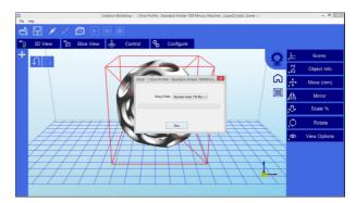
You can check again that the correct profile is being used and if not, you can select the correct one. Always click on the "Slice" button if you adjust the layout in any way.
