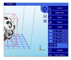
A model can be scaled (reduced or increased) by selecting it, and using the 'Scale' view to enter in a new scaler value. Press the tick button to re-scale your object.
