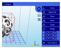
Rotating a model works in a similar way to moving a model. Simply select the model you want to work with, and use the X/Y/ Z +/- buttons to rotate the model by your specified degrees.
